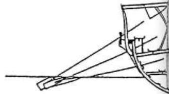
This drawing by the naval architect J F Coates shows the general arrangement of his reconstruction of a typical Athenian trireme. The hull is long, narrow and sits quite high in the water; the ram protrudes forward of the bow at the waterline. The oarsmen's seats are very close together and there is little space for carrying soldiers and supplies. (J F Coates)
