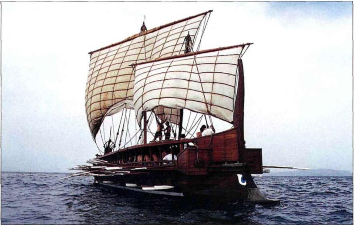
This photo is of the Hellenic naval vessel *Olympics*, a working reconstruction of an Athenian trireme. Such warships routinely used their sails for long voyages, but they were propelled by their oars alone during battles: the masts were removed and stored on land. Some triremes were used to transport soldiers and a few were even converted to carry up to 30 horses. (Ancient Art and Architecture)
